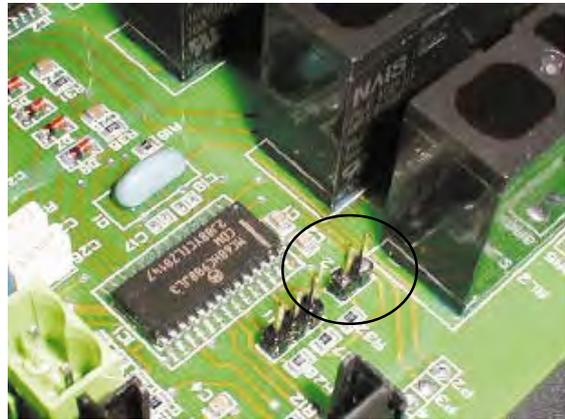
Manual reset mode and water purge out for a short time only at beginning of every harvest cycle plus a full water purge every six cycles - Recommended for normal/hard water - JUMP IN TWO contacts of J1
