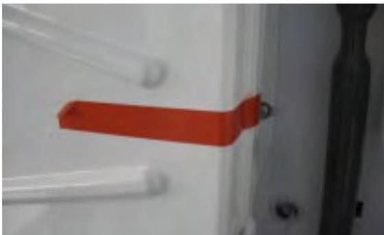
Remove first the ice deflector/evaporator cover then the masking tape from the ice thickness sensor.
