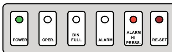
The fifth **Red LED** is **ON STEADY: TOO HI DISCHARGE PRESSURE > 33 bar (460 PSI)**
