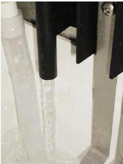
3. Water is coming into the water through the Water Inlet Solenoid Valve till the water reservoir is filled up to the maximum level controlled by a Water Level Sensor.
