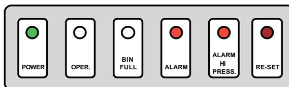
Both the last two **Red LED** are **ON STEADY: Condenser Sensor OUT OF ORDER.**
