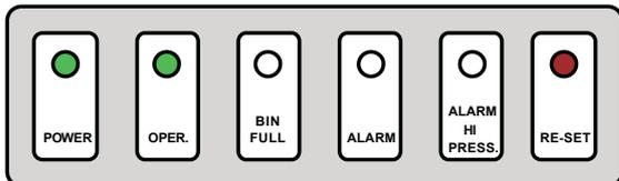
The **Green LED** of machine in operation is energized too, **blinking fast for 40 seconds**.
